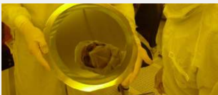
Markus Wimplinger shows Françoise von Trapp a 300mm bonded wafer on tape carrier.
